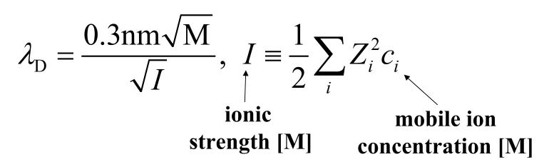
$\lambda_D$  is how much free charges can be separated (local breakdown of electro-neutrality) spatially by thermal fluctuation energy.
