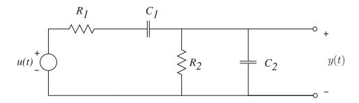
Assume that  $R_1 = R_2 = 2 \Omega$ ,  $C_1 = 0.2 \text{ F}$ , and  $C_2 = 0.3 \text{ F}$ .
