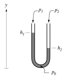
We now pick  $p_0$  to be the pressure at some point of the tube (at the bottom for instance), and apply equation (2) to each leg of the tube.
