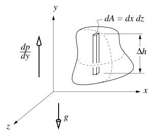
where dp/dy has been replaced by  $-\rho g$  using the Hydrostatic Equation (1), and the volume of the infinitesimal volume is  $\Delta h \, dA = d\mathcal{V}$ . Integrating the last equation above then gives the total buoyancy force on the object.
