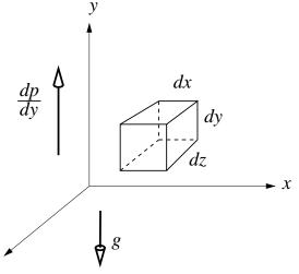
If the fluid element is at rest, the net force on it must be zero. For the vertical y-force in particular, we have
