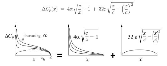
Define  $x_h$  as the location of the flap hinge, so the flap extends from  $x = x_h$ , to the trailing edge at x = c. The corresponding  $\theta$  locations are  $\theta = \arccos(1-2x_h/c) \equiv \theta_h$ , and  $\theta = \pi$ , respectively. The load/span and moment/span coefficients on the flap hinge can now be computed by integrating the pressure loading.
