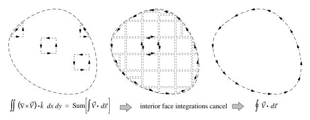
Figure 6: Summation of curl over interior of a finite circuit
