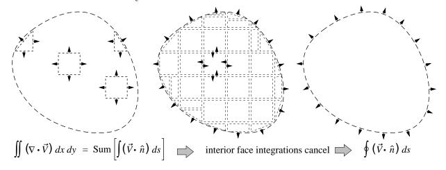
Figure 5: Summation of divergence over interior of a finite CV
