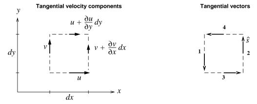
Figure 4: Infinitesimal CV with tangential velocity components.
