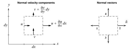
Figure 2: Infinitesimal CV with normal velocity components.
