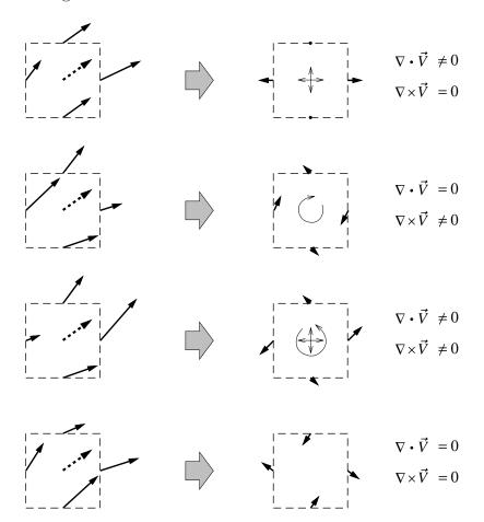
Figure 8: Example velocity distributions around a CV or circuit.
