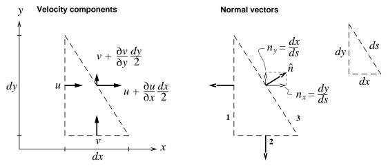
Figure 3: Infinitesimal triangular Control Volume.
