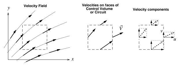
Figure 1: Velocity field and Control Volume.
