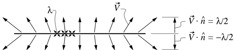
The normal velocity is then simply a constant  $\lambda/2$  directed outward. But if any other singularity or freestream is present, this additional velocity will be superimposed on each side of the sheet. For example, if the sheet is immersed in a freestream, we will have
