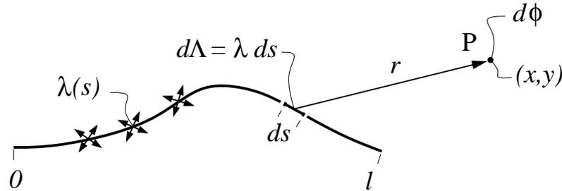
The potential of the entire sheet at point P is then obtained by integrating the infinitesimal contributions all along the sheet.
