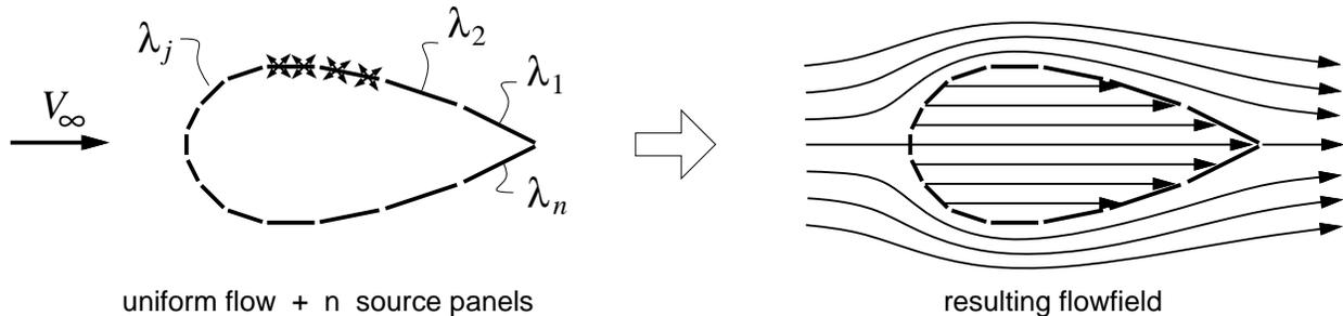
This use of source sheets in this manner to represent a flow is the basis of the *panel method*, which is widely used to compute the flow about aerodynamic bodies of arbitrary shape. The approach presented here is actually suitable only for non-lifting bodies such as fuselages. For airfoils, wings, and other lifting bodies, vortices must be added in some form to enable circulation to be represented. This modification will be treated later.
