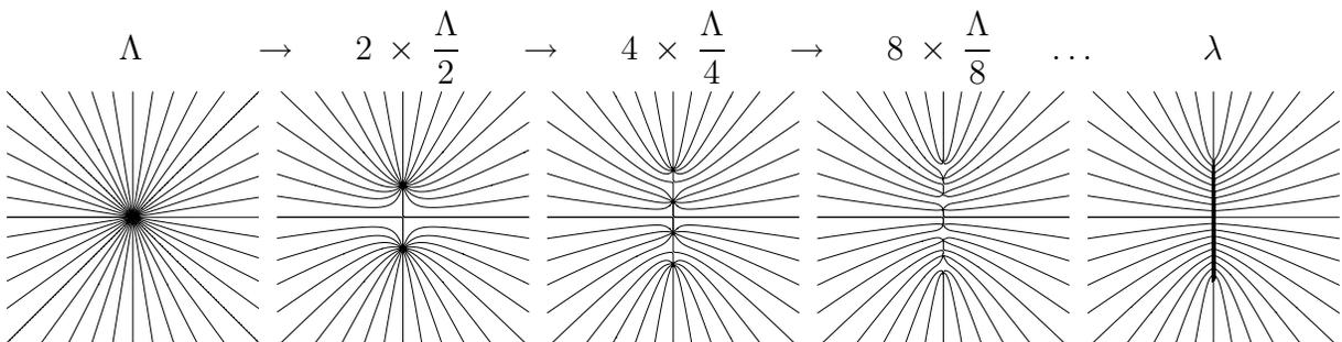
The units of  $\Lambda$  are  $\text{length}^2/\text{time}$ , while the units of  $\lambda$  are  $\text{length}/\text{time}$  (or velocity). Note that the total source strength is not changed in this process.
