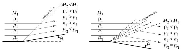
normal shock, and across an expansion fan they are in the opposite direction. One important difference is that  $p_o$  decreases across the shock, while the fan is isentropic, so that it has no loss of total pressure, and hence  $p_{o_2} = p_{o_1}$ .
