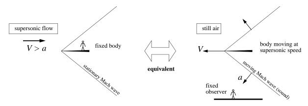
The angle  $\mu$  of a Mach wave relative to the flow direction is called the *Mach angle* It can be determined by considering the wave to be the superposition of many pulses emitted by the body, each one producing a disturbance circle (in 2-D) or sphere (in 3-D) which expands at the speed of sound a. At some time interval t after the pulse is emitted, the radius of the circle will be at, while the body will travel a distance Vt. The Mach angle is then seen to be
