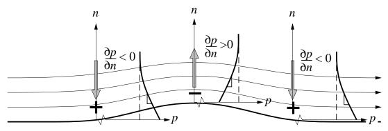
The curvature/pressure-gradient relation also indicates the pressures which can be expected on the surface of a body such as an airfoil. Examination of the streamline curvatures indicates that for a symmetric airfoil at zero angle of attack, higher pressure is expected at the leading and trailing edges, while lower pressure is expected along the sides.
