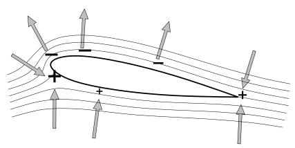
The actual surface pressure force vectors  $-C_p\hat{n}$  are shown for the NACA 0015 airfoil, at  $\alpha = 0^{\circ}$  ( $c_{\ell} = 0$ ), and  $\alpha = 10^{\circ}$  ( $c_{\ell} = 1.23$ ). The  $C_p(x)$  distributions are also shown plotted.
