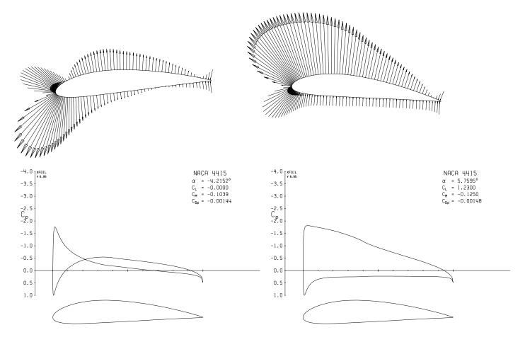
The leading edge spike at the high angle of attack is indeed reduced considerably. The low angle of attack case now has a "negative" spike on the bottom surface, but this is much weaker and appears tolerable.
