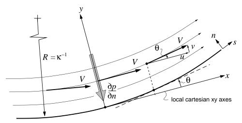
To determine how the pressure varies normal to the surface, we align local xy axes tangent and normal to the surface, and employ the y-momentum equation, with the viscous forces neglected.
