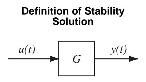
The LTI system *G* is Bounded Input / Bounded Output (BIBO) stable if every bounded input u(t) produces a bounded output y(t).
