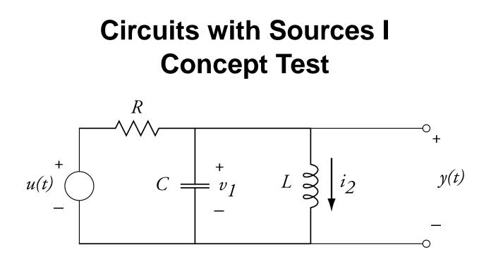
For the circuit above, take  $v_1$  and  $i_2$  to be the state variables. Find the differential equation for the state  $i_2$ .
