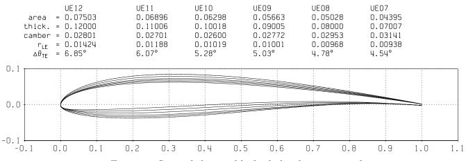
Figure 1: Six airfoils suitable for light electric aircraft.
