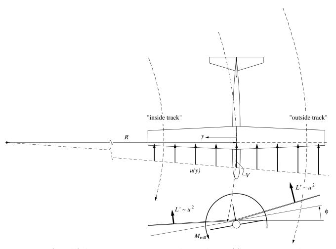
Figure 8: Curved flight path in a turn causes a relative velocity u(y) variation across the span, which produces an inward rolling moment from the resulting lift imbalance.
