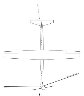
Figure 9: Outward roll moment from ailerons cancels inward roll moment from curved flight path, thus maintaining a constant bank angle.
