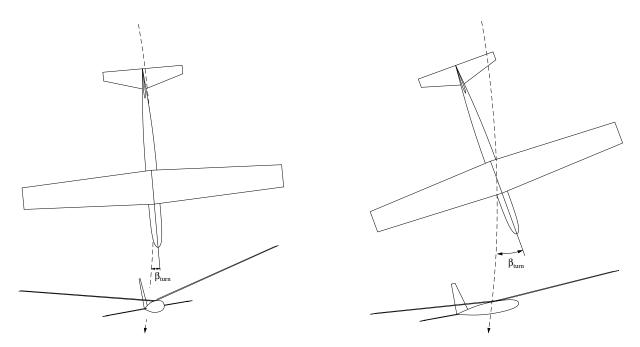
Figure 10: Outward roll moment from sideslip angle cancels inward roll moment from curved flight path, thus maintaining a constant bank angle. Smaller dihedral requires larger sideslip.
