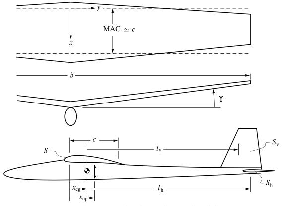
Figure 1: Lengths, areas, and angles used in simple stability criteria.
