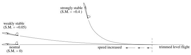
Figure 3: Pitch-up behavior from an airspeed increase, for large and small Static Margin.
