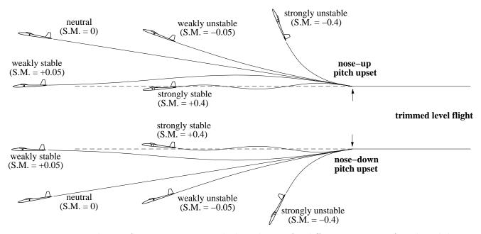
Figure 2: Natural aircraft responses to a pitch disturbance, for different amounts of pitch stability.
