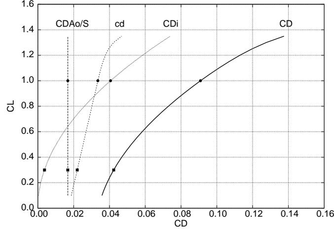
Figure 1: Drag polar and drag polar components for electric sport aircraft.  $AR = 9.0$
