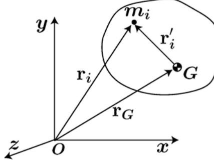
$$T = \sum_{i=1}^n \frac{1}{2} m_i (\mathbf{v}_G + \dot{\mathbf{r}}'_i) \cdot (\mathbf{v}_G + \dot{\mathbf{r}}'_i) = \frac{1}{2} m v_G^2 + \frac{1}{2} \omega \int_m r'^2 dm = \frac{1}{2} m v_G^2 + \frac{1}{2} \omega^2 I_G. \quad (25)$$
