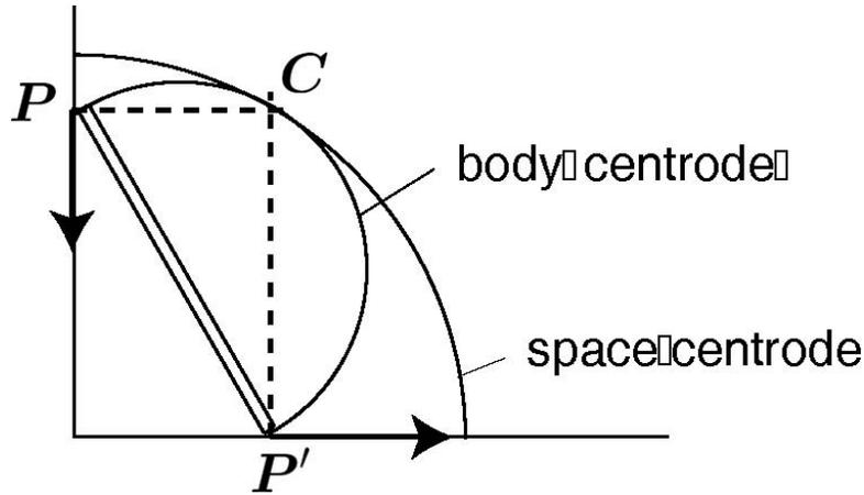
From this example, it should be clear that although we think about the instantaneous center of rotation as a point attached to the body, it need not be a material point. In fact, it can be a point “outside” the body. It is also possible to consider the instantaneous center of acceleration as the point at which the instantaneous acceleration is zero.
