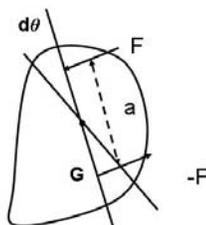
If  $M$  is constant, the work is simply  $W_{1-2} = M(\theta_2 - \theta_1)$ . In other words, the couples do work which results in the kinetic energy of rotation.
