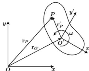
In order to determine the motion of a point  $P$  in the body, we consider a second set of axes  $x'y'$ , always parallel to  $xy$ , with origin at  $O'$ , and write,
