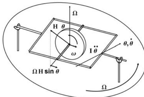
The unsteady term is  $I_0\ddot{\theta}$ , where  $I_0$  is the moment of inertia of the disk about the axis perpendicular to its spin axis; the vector is in the horizontal direction. The horizontal component of the angular momentum of the disk is  $I\omega\sin\theta$ , where  $I$  is the moment of inertia of the disk about its axis of rotation. The rate of
