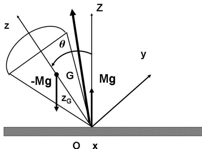
Initially, we shall not assume steady motion, but will develop Euler's equations in the Euler angle variables  $\psi$  (spin),  $\phi$  (precession) and  $\theta$  (nutation).
