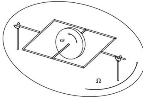
Consider the gyroscope shown in the figure. It is free to spin about its axis with angular velocity  $\omega$ . It is attached to a gimbal which is free to rotate about the support as sketched. The entire apparatus is mounted on a turntable rotating with angular velocity  $\Omega$ , where  $\omega \gg \Omega$ . If we can measure the orientation of the axis of rotation of the disk relative to the turntable mount, we could possibly use this as an instrument. What does it measure?
