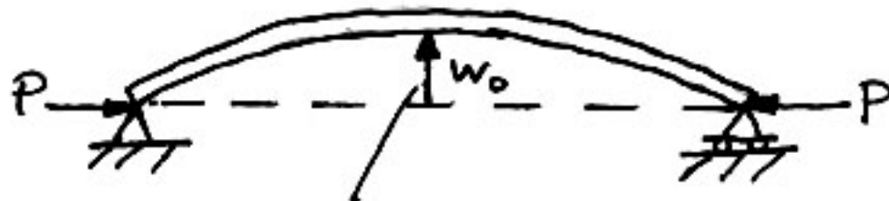
Figure 16.12 Representation of column with initial imperfection
