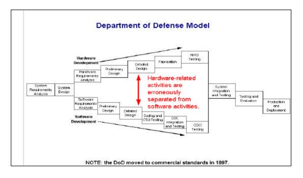
Figure 6 - DoD Model for System Development [43]
