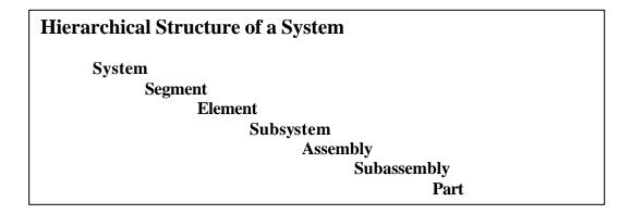
Figure 1 - Hierarchical Structure of a Generic System (Derived from [10])
