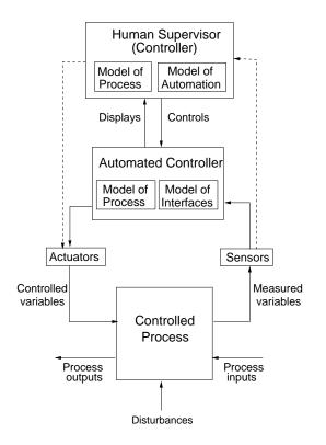
Figure 3: A typical control loop and the process models involved.
