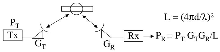
L = free space loss, d = distance between Tx and Rx  $\lambda =$  signal wavelength
