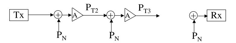
• A repeater simply amplifies the signal to make up for attenuation
