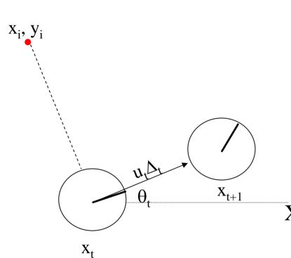
Position of robot is represented as a triple consisting of its  $x_t$ ,  $y_t$  components and its heading  $\theta_t$ :
