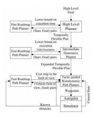
Figure 2: Overall Architecture of the Activity / Path Planner
