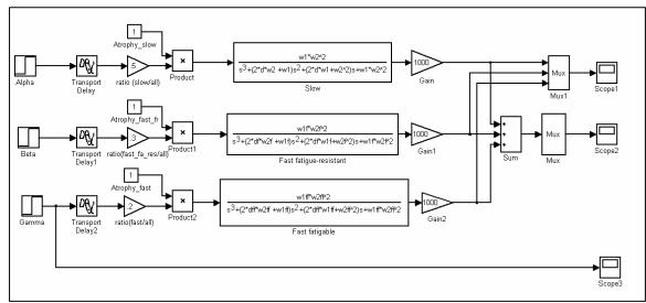
Figure 4.1 Simulink model that increases overall number of fibers to 1000
