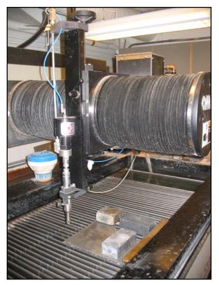
Figure 40 Setup of part to cut with water jet cutter
