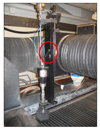
Figure 44 Location of lever to lock-in desired height of water jet cutter nozzle
