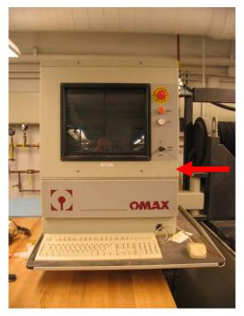
Figure 34 Location of power switch to water jet system
