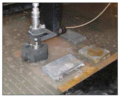
Figure 47 Water jet cutter in operation
