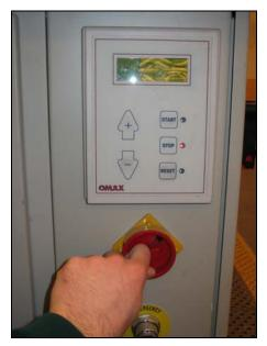
Figure 35 Turning on/off power to water jet cutter
