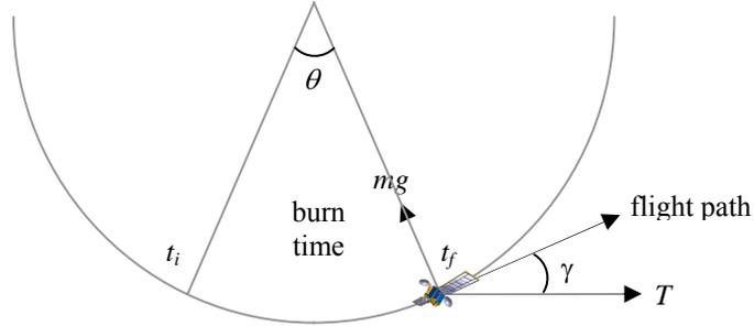
Figure 1. Forces during finite burn.
