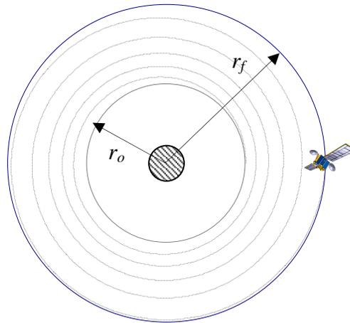
Figure 2. Low thrust spiral orbit.
