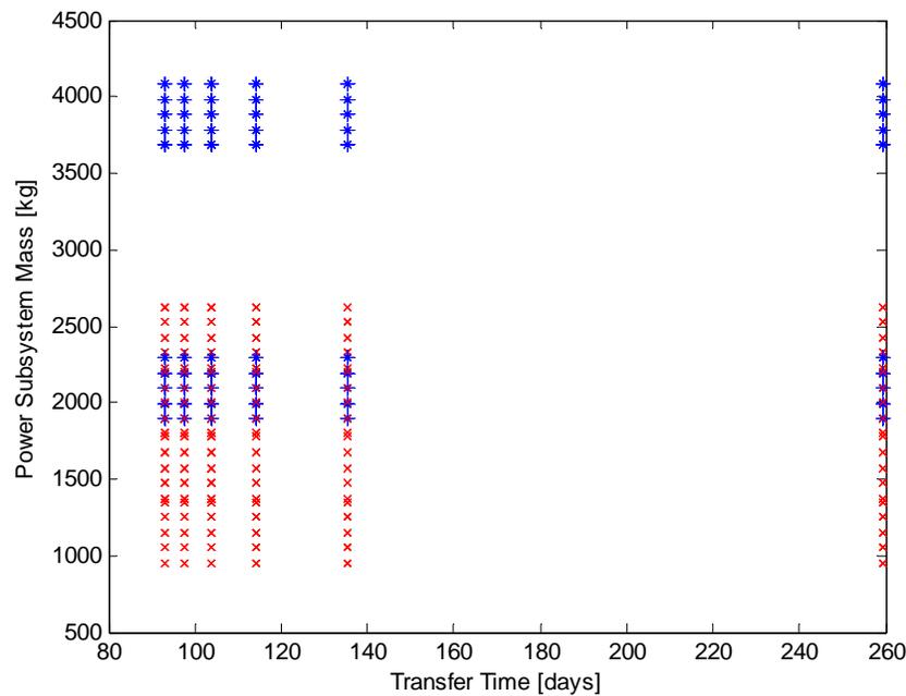
**Figure 8. Power subsystem mass for transfer orbits ranging from Hohmann transfer to a high energy transfer with 2.5 AU semi-major axis. Blue signifies the use of RTG and red signifies the use of solar array as a power source.**
