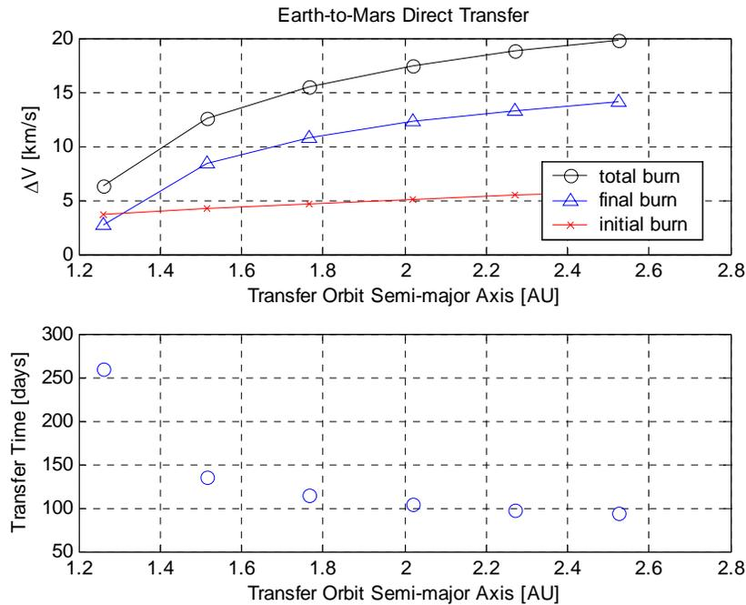
Figure 5. Transfer  $\Delta V$  and transfer time as a function of transfer orbit semi-major axis.
