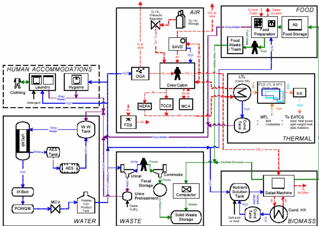
Figure 3. Schematic diagram of Environment Control and Life Support System for a Mars Transfer Vehicle using ALS Technology [Stafford, 2001]
