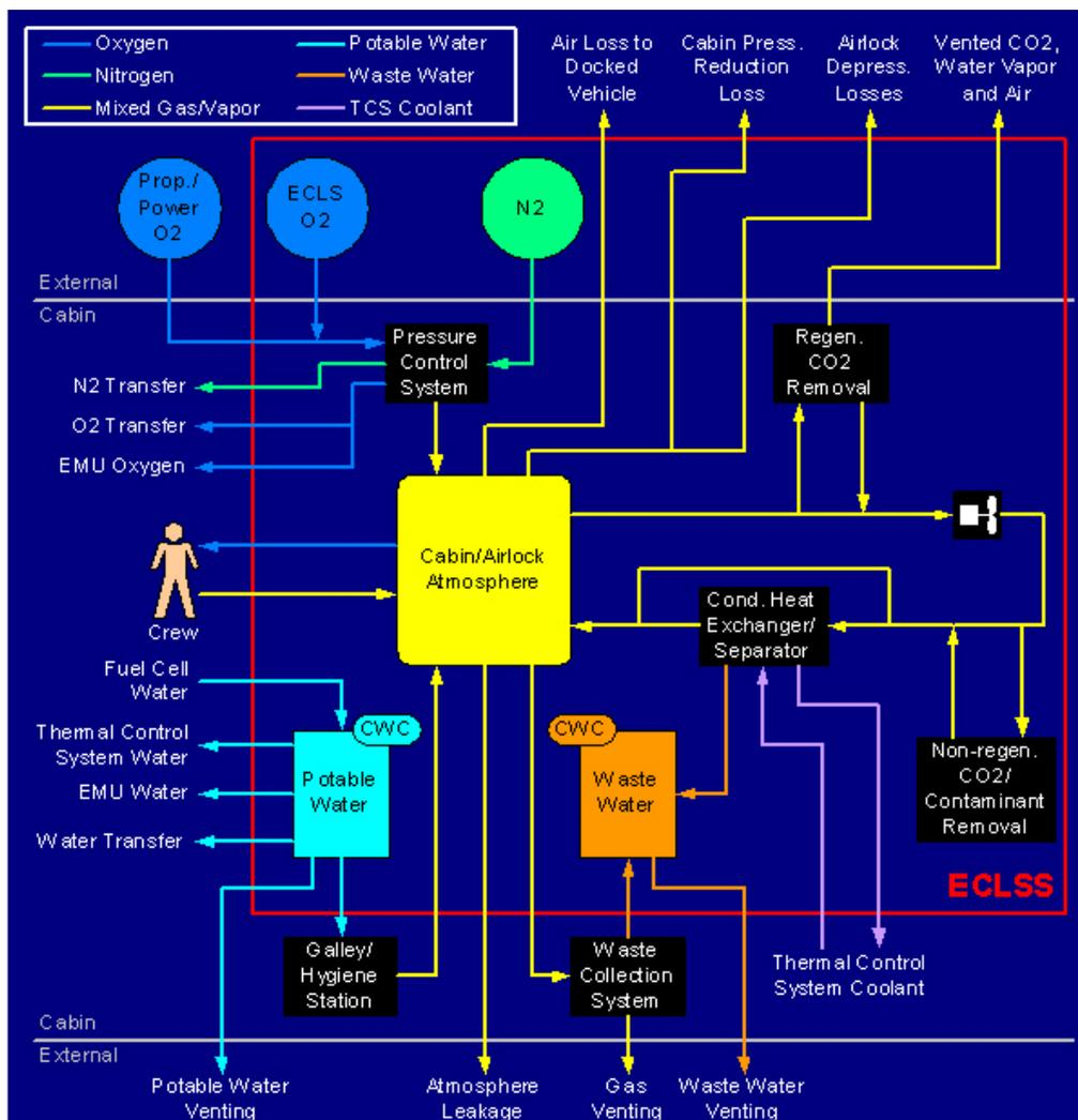
Figure 1. Schematic diagram of Environment Control and Life Support System [Lawson, 2003]
