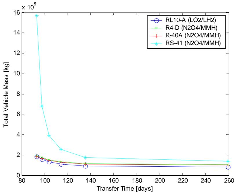
**Figure 9. Total vehicle mass for transfer orbits ranging from Hohmann transfer to a high energy transfer with 2.5 AU semi-major axis with respect to various propulsions system.**
