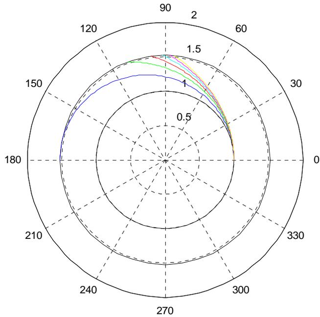
Figure 6. Transfer orbit trajectories ranging from Hohmann transfer to a high energy transfer with 2.5 AU semi-major axis. Note that the radius is in AU.
