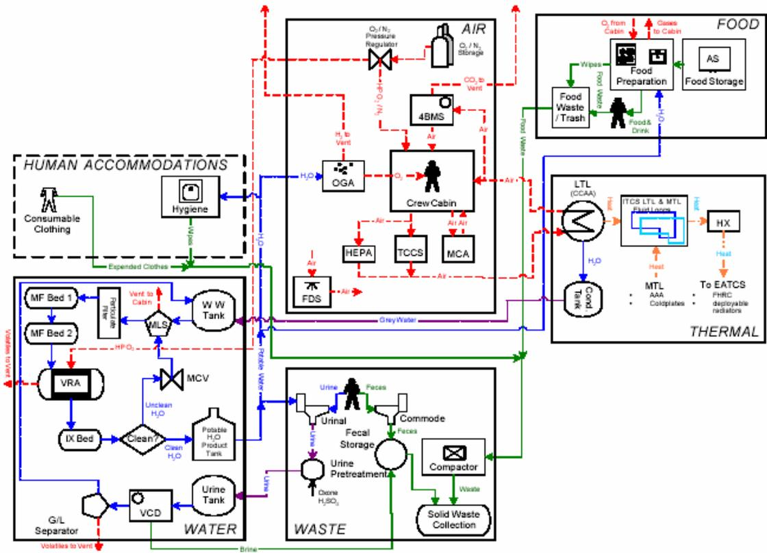
Figure 2. Schematic diagram of Environment Control and Life Support System for a Mars Transfer Vehicle using ISS-Baseline Technology [Stafford, 2001]
