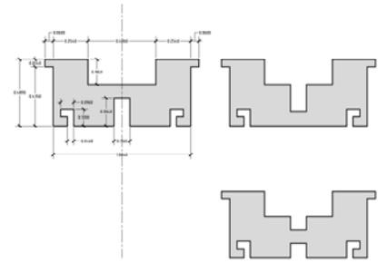
Figure 6.0 *Design description of joint*
