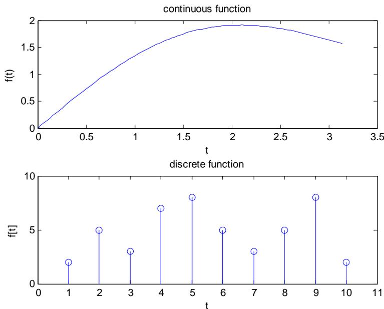
The distinction is very important to us because when we use computers to numerically perform mathematical operations we are confined to dealing with the properties of discrete numbers. That is because typical computers are built with digital logic dealing with ultimately binary data. MATLAB can approximate a continuous
