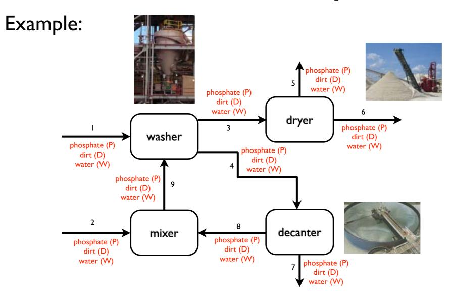
Stream 1 carries 1800 kg/hr P, 1200 kg/hr D and 0 kg/hr W Stream 2 carries 0 kg/hr P, 0 kg/hr D and 10000 kg/hr W Stream 3 carries 0 kg/hr D and 50% W into the washer Stream 4 carries 0 kg/hr P Stream 5 carries 0 kg/hr P and 0 kg/hr D Stream 6 carries 0 kg/hr D and 0 kg/hr W Stream 7 carries 0 kg/hr P, 95% of D into the decanter, 5% of W into the decanter Stream 8 carries 0 kg/hr P Stream 9 carries 0 kg/hr P
