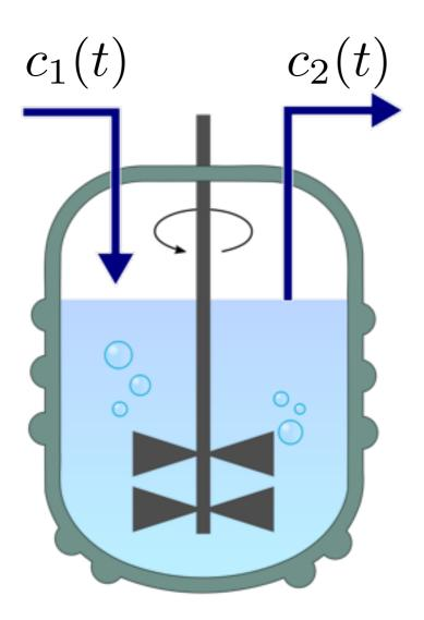
$$\frac{dc_2}{dt} = \frac{Q}{V} \left( c_1(t) - c_2(t) \right)$$
