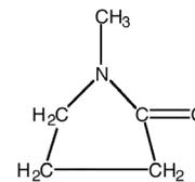
NMP is soluble in water but PES is not. Thus water extracts NMP from the exposed PES-NMP surface, rapidly concentrating the polymer and at the same time precipitating it as a skin, permeable to small molecules but not macromolecules. Water gradually diffuses through this skin and slowly precipitates the underlying PES-NMP, with the formation of micron-size columnar pores. The column-like structure mechanically supports the thin "permselective" skin. (See below micrographs)
