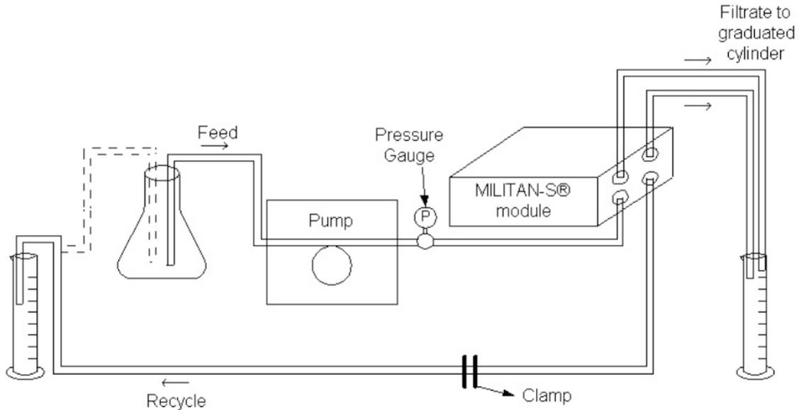
Figure 9: Final set up for permeability studies
