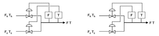
Each structure comprises two separate control loops; i.e., connections between a controlled and a manipulated variable. In the left figure, for example, if the flow rate is observed to change, the hot water valve will be adjusted. Changes in the temperature motivate adjustments to the cold water valve. The right figure makes the opposite pairings between CV and MV.
