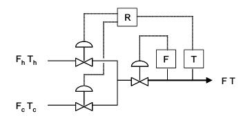
Alternatively, we could write a special-purpose controller algorithm (it would surely include material and energy balance equations!) that would accept two measurement inputs and compute two valve settings. Sometimes this extra effort in control design pays off in better process operation.
