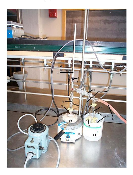
Figure 2. Apparatus used for Vacuum Distillation
