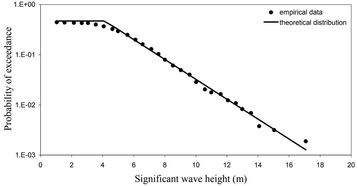
Figure 3: Annual probability of exceedance of significant wave height based on 1600 years of simulation.
