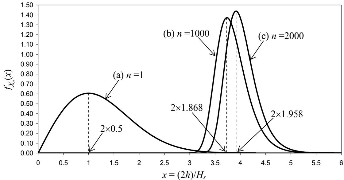
Figure 1: Probability density function,  $f_{X_n}(x)$ , of the maximum normalized height,  $X_n = (2H_n)/H_s$ , of  $n$  waves.
