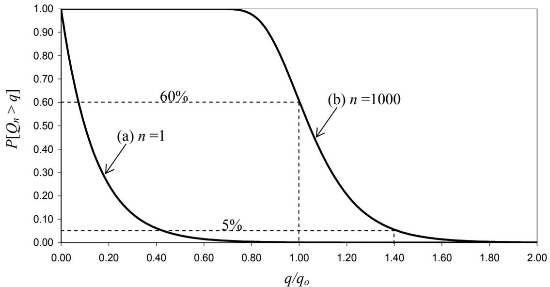
Figure 2: Exceedance probability  $P[Q_n > q]$  of the maximum load  $Q_n$  from  $n$  waves as a function of  $q/q_o$ , where  $q_o$  is the design load. The curves correspond to  $C = 2$  and design wave height  $h_o = 1.868H_s$ .
