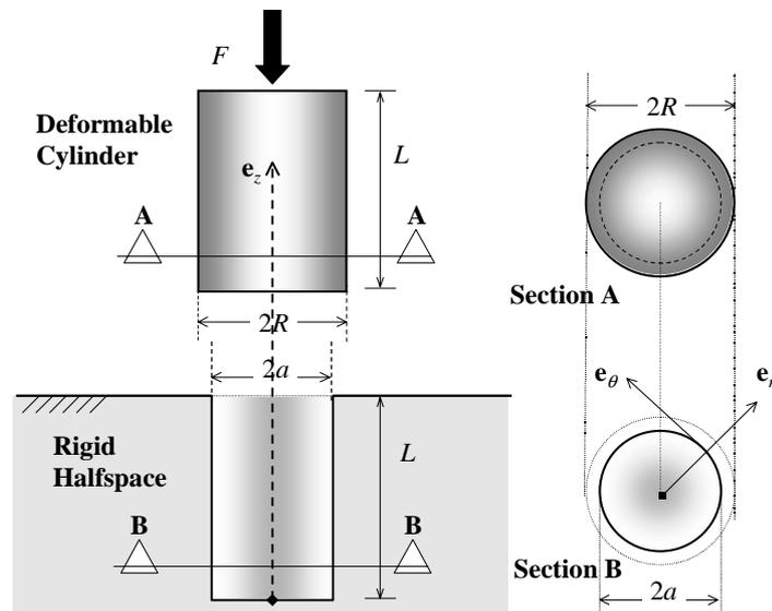
Deformable cylinder in a rigid halfspace.
