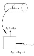
A closed can of soda is under pressure equivalent to that in an automobile tire. We measured the wall thickness in lab on Thursday to be 0.0025 inches. Estimate the axial stress  $\sigma_a$  and the hoop stress  $\sigma_{\theta}$ ? acting at a point in this closed, thin cylindrical shell, away from the ends. C
