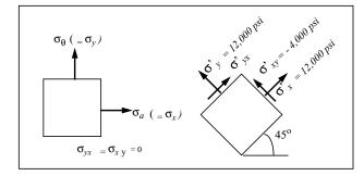
The same results could have been obtained without the use of Mohr's circle from the relationships which define the transformation of components of stress (in 2D) which appear on p. 118 in the text.
