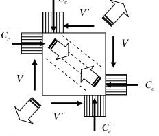
→  $V_c = C_c - V'$  = shear force transferred through concrete
