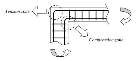
• Full strength of the bars can be developed if there is no bond failure.
