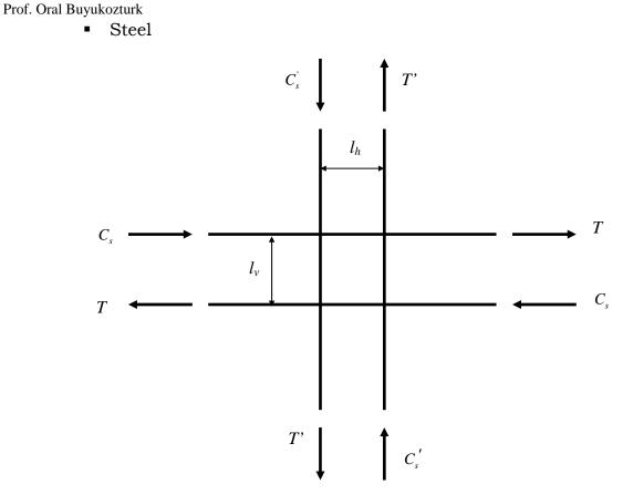
→  $V_s = C_s + T$  = shear force transferred through steel →  $u_0 = \frac{C_s + T}{l_h}$  and  $v_0 = \frac{C_s + T}{l_v}$
