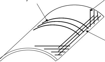
$N_{x\phi} = N_{\phi x}$  (mid-thickness) To accommodate diagonal Tensile stress associated with  $N_{x\phi} = N_{\phi x}$  at 45°.
