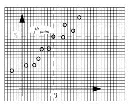
The aim now is to set m, the slope of our "best fit" line and b, its intercept with the y axis. The criteria we use is to minimize the "least square error" of the y coordinate. (This is not the only criterion that might be usefully applied. Can you think of another?) That is we seek to choose m and b to minimize the quantity
