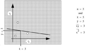
You might have expected another result, e.g., a line through the origin, passing through the point 1,1. But consider the criterion we applied: The error we minimize is proportional to the vertical distance between the data point and the line. Try computing the error of the best fit line and compare it with a line through 0,0 and 1,1.
