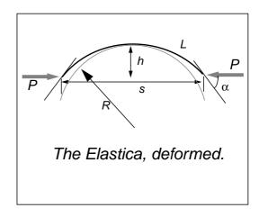
try of the deformed lamina. We present here only the essential results of the analysis; we defer a more complete presentation until later in the subject. The solution yields expressions for the height h and the span s in terms of two parameters, one related to the slope at the ends
