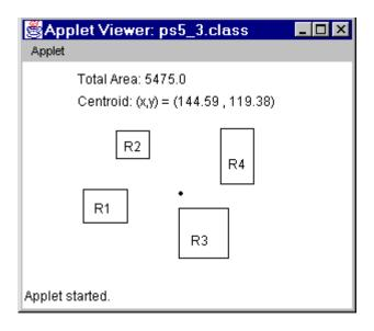
The centroid of a set of shapes is computed as the sum of the products of the area of each shape times its centroid coordinate  $(X_{ci} \text{ and } Y_{ci})$  divided by the total area of the cross-section. For example, the centroid  $(X_c, Y_c)$  of the following section is defined by the following formulas:
