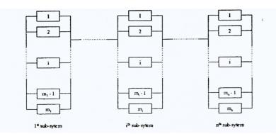
Schematic illustration of a parallel-series system
