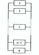
Schematic illustration of a parallel system
