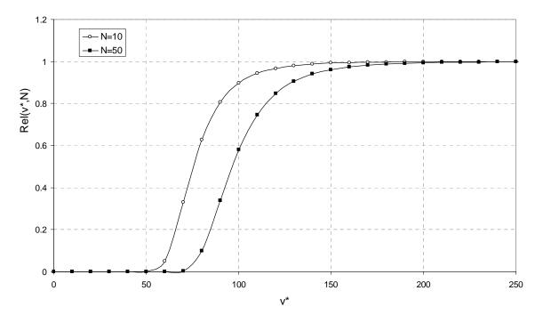
Figure 1: Reliability of a building in Boston against wind as a function of design wind speed  $v^*$ , for exposure periods of 10 and 50 years.
