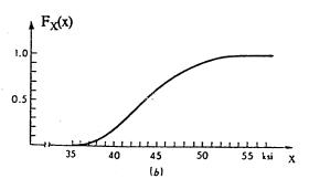
Example of PDF and corresponding CDF of a continuous random variable: steel-yield-stress. (a) Probability density function; (b) cumulative distribution function.
