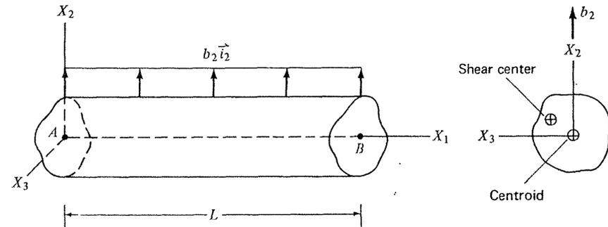
**Fig. E12-1****Twist About the Shear Center**
