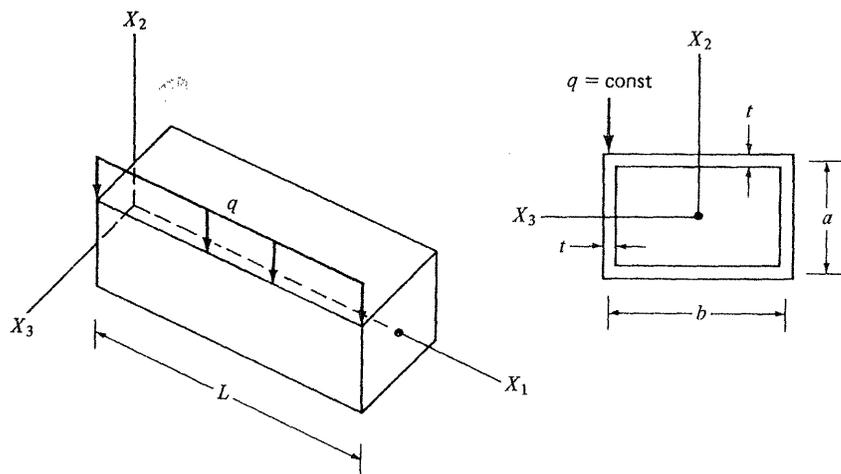
12-3. For the problem sketched, determine the complete solution by the displacement method.
