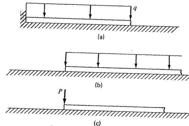
12-5. The formulation for the beam on an elastic foundation is based on a continuous distribution of stiffness; i.e., we wrote
