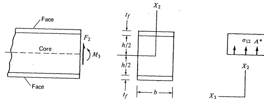
The shearing stress distribution is determined by applying the engineering theory developed in Sec. 11-7. Integrating the axial force-equilibrium equation over the area  $A^*$  and assuming  $\sigma_{12}$  is constant over the width, we obtain
