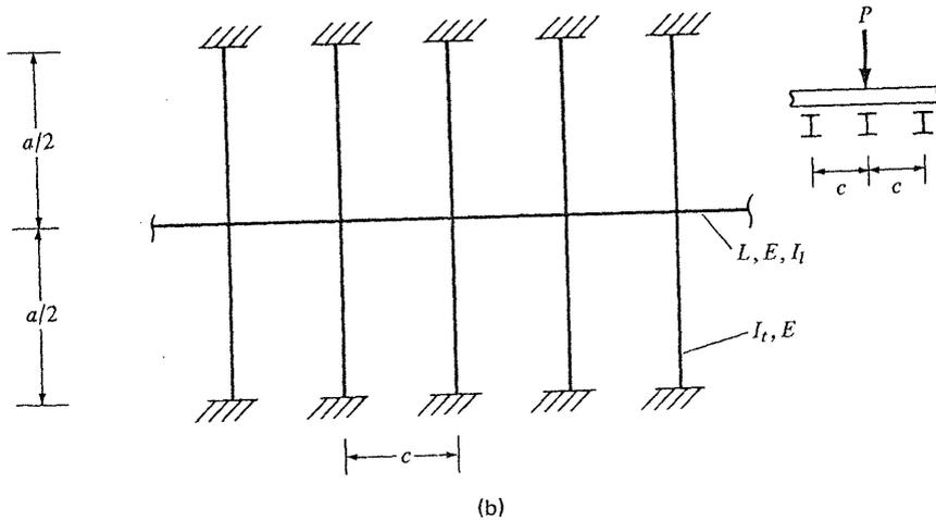
Consider the beam of part b, supported by cross members which are fixed at their ends. Following the approach outlined above, determine the distribution of force applied to the cross members due to the concentrated load,  $P$ .
