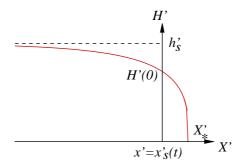
Figure 2.4.2: Matching the near-field and far-field at the front by preserving mass.
