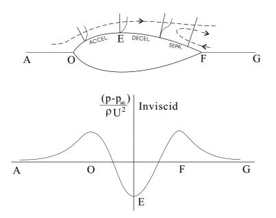
Figure 3.4.1: Pressure variation along the surface of a a blunt body
