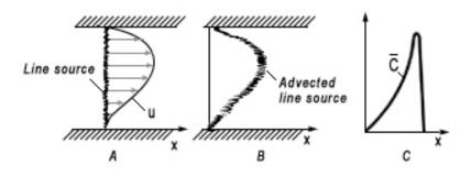
Figure 4.6.1: Initial stage of convective diffusion of a die streak. From Fischer et al.
