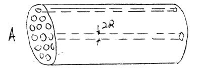
Figure 6.1.2: A one dimensional model of porous medium
