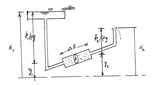
Figure 6.1.1: Darcy's experiment for seepage flow
