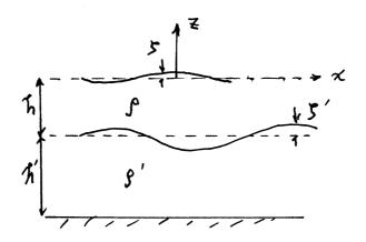
Figure 7.8.1: A two-layered sea of contant depth.
